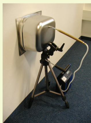
Figure 1. Emission cell against the wall
